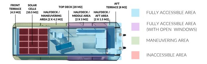
ON THE TOP DECK, A USABLE AREA REDUCED BY THE PHOTOVOLTAIC PANELS IS LOCATED. THE COMBINED SPACE OF THE TERRACES [32.5M2] MAKES A LARGE, FULLY ACCESSIBLE AREA. THE HALF-DECK AREA IS ALSO AVAILABLE IN 100%, BUT ITS USEFULNESS INCREASES FROM THE AFT - AS AN EXTENSION OF THE AFT TERRACE, ENLARGEMENT OF THE LIVING ROOM AFTER OPENING THE WINDOWS TO THE HALF-DECKS USED IN MANEUVERING SITUATIONS.
